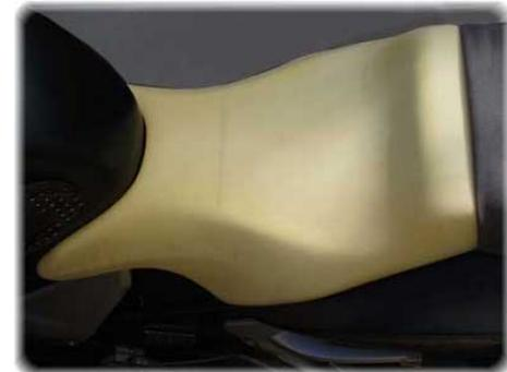
**2** These pictures outline the basic plan of attack. The key changes shown here are reducing the forward pitch, increasing cradle and, increasing the length of the driver's platform to give taller riders a bit more forward-backward room.
