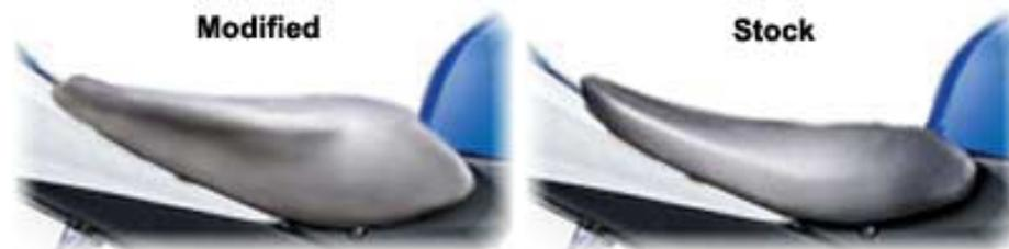
One part of the seat that helps decrease the obnoxious forward slide of so many stock seats is a well-shaped "nose." The pictures below show a Suzuki Haybusa stock seat (left) and a [Corbin](#) Hayabusa replacement seat with a more pronounced nose. The nose not only prevents the rider from sliding forward as much, but also helps distribute weight across the seat, thereby removing some pressure from the sitting bones.
