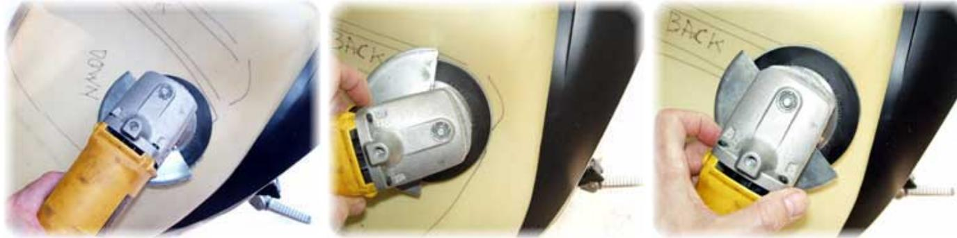
Always use eye protection and a filter mask when grinding foam. Grinding foam can kick up a lot of dust that can irritate your eyes and lungs.
