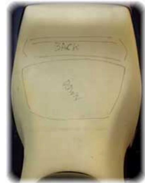
**3** Carefully grind down the areas of the stock foam that you've identified. Use very light pressure with the grinder, as it easily cuts through and takes off foam. Use longer strokes where possible, instead of working the grinder in one small area. Never push the grinder into the foam in the direction of its rotation; instead, pull it towards you, gently "sweeping" away the foam you want to remove.
